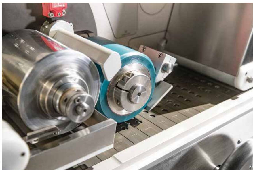
Photo 1: The printer's continuous-motion, multiple-lane conveyor feed system features carrier bars with pockets that precisely position the tablets and expose their top surfaces for printing.
